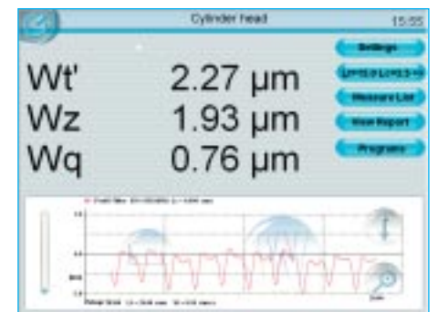
Result display Waviness parameters and waviness trace
